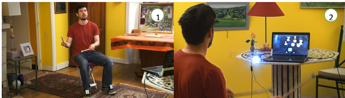
Figure 1: (1) Users hit the air to hit the invisible drums. (2) Users can see the position of the sticks relative to the drums on the computer screen.
